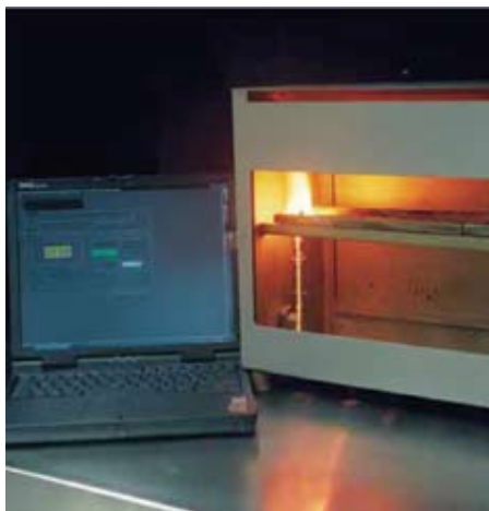
4 Test chamber for determining horizontal rate of combustion
